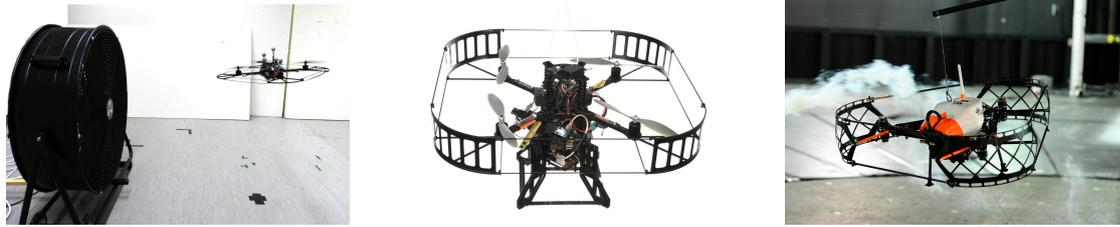
(a) AscTec Hummingbird. Copyright © 2014 IEEE [141, 137, 138, 141]. (b) AscTec Pelican with modular stereo vision based navigation system. Copyright © 2013 IEEE [123, 138]. (c) DLR Ardea coaxial hexacopter custom developed and built for the wind tunnel experiments in this thesis. Copyright © 2016 IEEE [140, 139].
