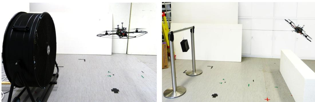
(a) Hovering in a 3 m/s turbulent wind stream, (b) Hovering with a constant side force produced by a fan with 70 cm diameter by a suspended 6 N weight
