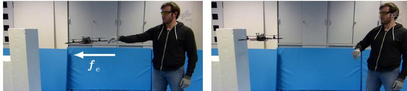
(b) Video stills of an interaction experiment. The human pushes the robot, which causes a collision. The secondary collision can be recovered from safely because the interaction controller amplifies the collision force; as a result, the robot bounces away from the obstacle.
